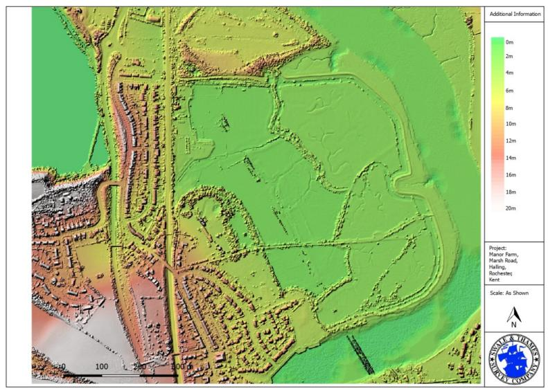
Figure 12: Elevation overlaying DSM LIDAR
